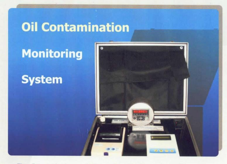
The oil contamination monitoring system offered by us is used for on-line measurement of contmination in Hydraulic oil and gives direct output in terms of CLASS OF COTAMINATION as per ISO 4406 or NAS 1638.
